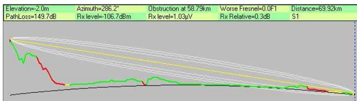
Figure 2. A profile plot of a particular radio link.
